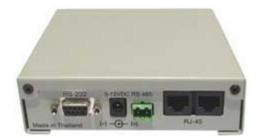
Figure 2H: Rear of TCPIP 232 Adapter
